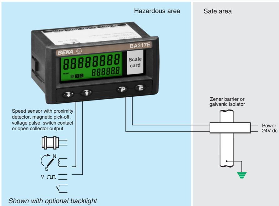
The **BA317E** is a third generation intrinsically safe tachometer that has similar functions as the BA318E, but is housed in a smaller 96 x 48mm DIN enclosure. The tachometer is easy to use and can be configured on-site to operate with a magnetic pick-off, switch contact, proximity detector, open collector or voltage pulse sensor. A slide-in scale card simplifies identification and international intrinsic safety certification permits worldwide installation.
