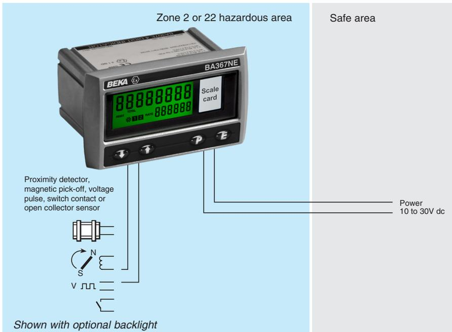
The BA367NE has a rugged stainless steel enclosure with Ex nA and Ex tc certification allowing it to be safely installed in an Ex n or Ex tc panel enclosure located in Zones 2 and 22, without the need for Zener barriers or galvanic isolators. The counter is easy to use and can be configured on-site to operate with a wide variety of sensors. A slide-in scale card simplifies identification.
