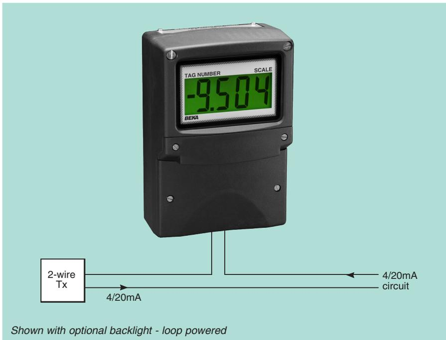
The **BA504E loop powered 4/20mA indicator** is a fourth generation field mounting instrument that is electrically and mechanically compatible with the earlier BA504D. It has a much larger full 4 digit display and guaranteed performance between -40 and 70°C. Like its predecessor, the BA504E is housed in a robust IP66 enclosure with a separate terminal compartment.
