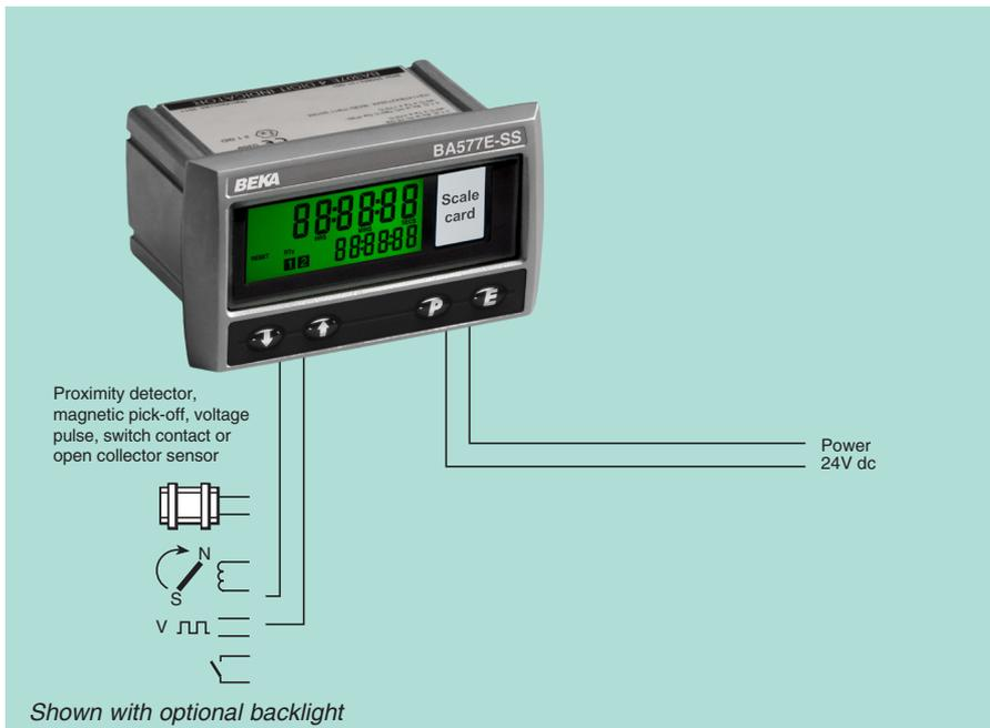
The **BA577E-SS** is a rugged general purpose instrument that may be configured as a Timer or as a Clock. Housed in a 316 stainless steel enclosure with a 10mm thick toughened glass window, it has IP66 front of panel protection and is suitable for use in hostile and marine environments, or where the front of the instrument is likely to be impacted.
