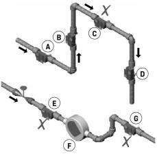
In order to prevent cavitation the back pressure (the pressure at the flow sensor outlet) at ULTRAFLOW® must be min. 1.5 bar at  $q_p$  and min. 2.5 bar at  $q_s$ . This applies to temperatures up to approx. 80 °C.
