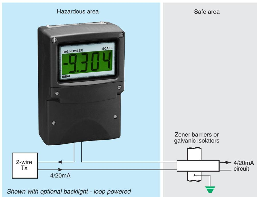
The **BA304E loop powered 4/20mA indicator** is a fourth generation field mounting instrument that is electrically and mechanically compatible with the earlier BA304D. It has a much larger full 4 digit display and guaranteed performance between -40 and 70°C. Like its predecessor, the BA304E is housed in a robust IP66 enclosure with a separate terminal compartment.
