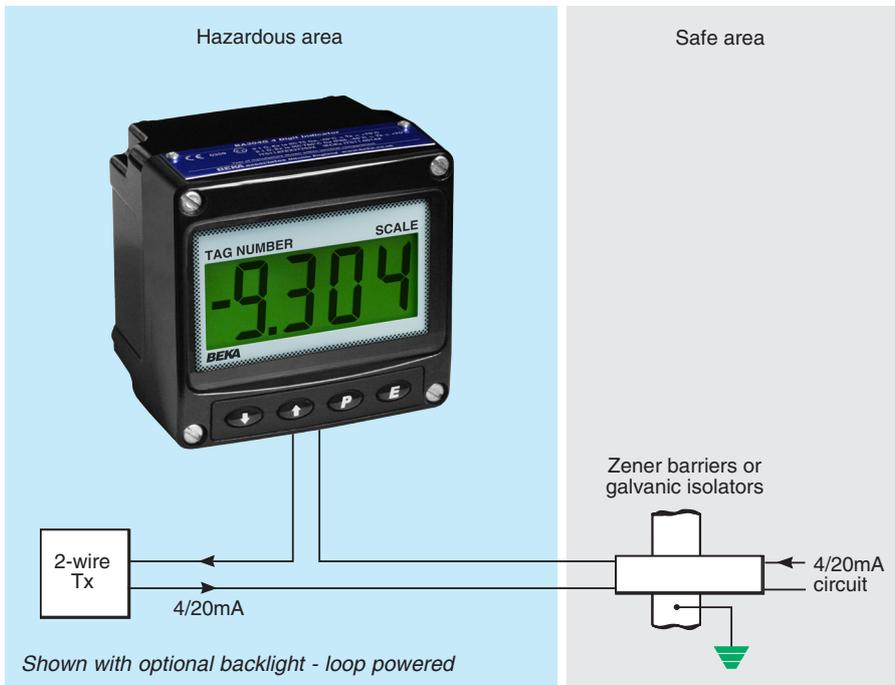
The **BA304G loop powered 4/20mA** indicator is a new field mounting instrument that supersedes the well established BA304C. It is electrically and mechanically compatible with the earlier model but has a much larger full 4 digit display and guaranteed performance between  $-40$  and  $+70^{\circ}\text{C}$ . Like its predecessor, the BA304G is housed in a robust IP66 enclosure which may be surface or pipe mounting.
