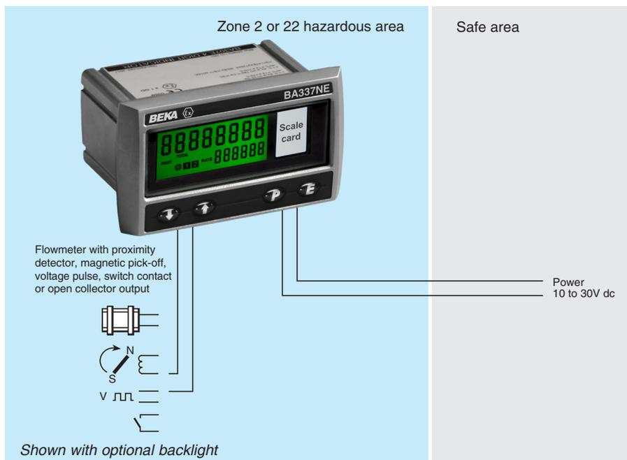
The **BA337NE** rate totaliser has a rugged stainless steel enclosure allowing it to be safely installed in an Ex n or Ex tc panel enclosure located in Zones 2 or 22 without the need for Zener barriers or galvanic isolators. The rate totaliser is easy to use and can be configured on-site to operate with flowmeters having a wide variety of pulse outputs. A slide-in scale card simplifies identification.
