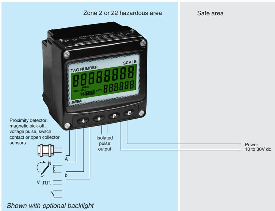
The **BA384NG** is a two input, field mounting, Ex nA and Ex tc certified rate totaliser that can simultaneously display the total flow and rate of flow of either flowmeter, or the sum or difference of the two. The BA384NG is easy to use and each input can be individually configured on-site to operate with flowmeters having a variety of pulse outputs. A slide-in scale card simplifies identification and international certification permits worldwide installation.
