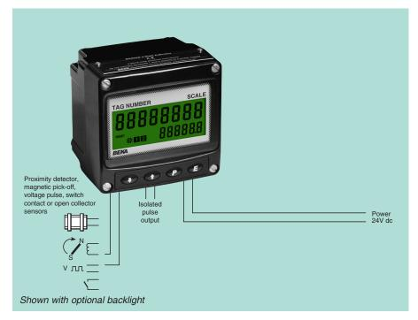
The BA514G is a third generation, general purpose field mounting tachometer housed in a compact IP66 GRP enclosure. The tachometer is easy to use and can be configured on-site to operate with a magnetic pick-off, switch contact, proximity detector, open collector or a voltage pulse sensor.
