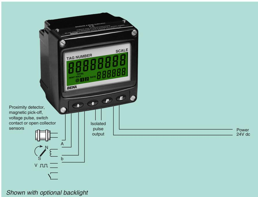
The **BA584G** is a two input, general purpose field mounting rate totaliser that can simultaneously display the total flow and rate of flow of either flowmeter, or the sum or difference of the two. The BA584G is easy to use and each input can be individually configured on-site to operate with a flowmeter having a variety of pulse outputs. A slide-in scale card simplifies identification.
