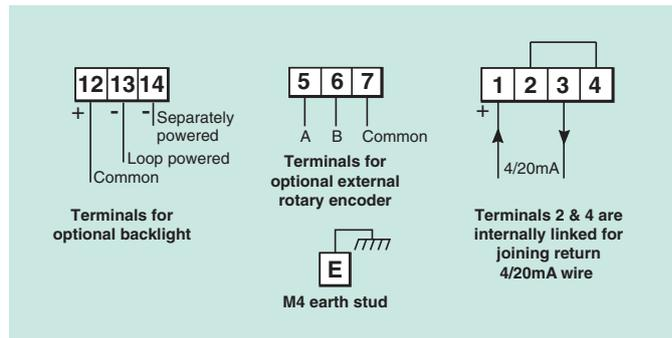
External encoder BA490 panel mounting rotary quadrature encoder which may be located up to 1m away from the BA627E-SS. See separate datasheet.
