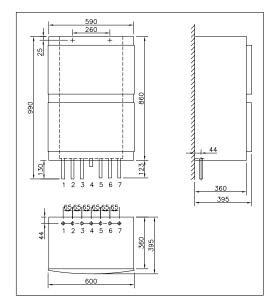
Internal installation and district heating\* pipe connections must be made by means of flange, thread or welding connections.
