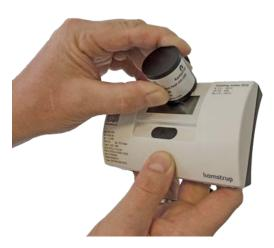
In connection with prolonged data readings, reading of data loggers, or if you want the optical reading head to be retained on the meter for other reasons, you can use a transparent holder, which is clicked onto the meter.
