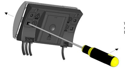
When the two mechanical locks have been released, remove the top cover from the base.
