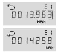
Example of display reading if the meter is configured for "flow sensor in inlet pipe"
