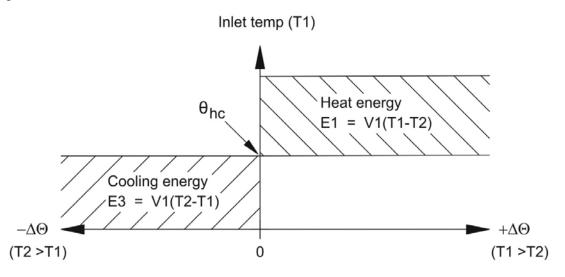
If current T1 exceeds or equals  $\theta_{hc}$ , only heat energy can be measured. If current T1 is lower than or equals  $\theta_{hc}$ , only cooling energy can be measured.
