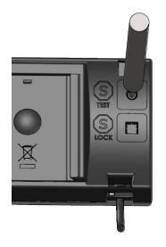
In order to access test mode the "TEST" seal S on the back of the meter must be carefully broken with a screwdriver and the contact points behind the seal short-circuited with short-circuit pen type 66-99-278.
