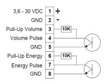
When Pulse Interface type 66-99-143 is connected to power supply or battery, the unit is placed on the meter, and the meter is in test mode, the following pulses are transmitted:
