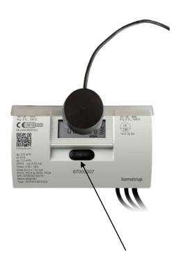
Start up METERTOOL HCW, press the button on the calculator and click "Connect" in METERTOOL HCW.
