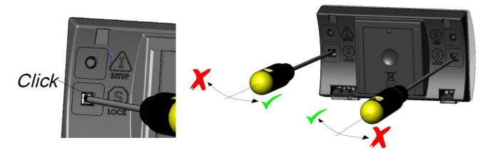
The seals are gently broken using a screwdriver.
