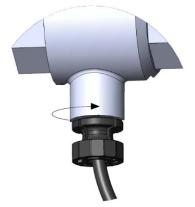
Fasten the plastic coupling manually. The use of tools is not permitted.
