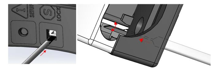
Close-up illustration of locking function being released.
