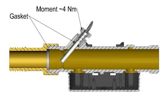
Mounting of couplings as well as temperature sensor mounted in MULTICAL<sup>®</sup> 302 flow sensor.
