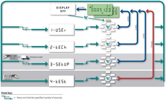
From the three top loops the meter automatically reverts to energy (heat energy or cooling energy, depending on the meter's configuration) 4 min. after the last activation of the push-button.
