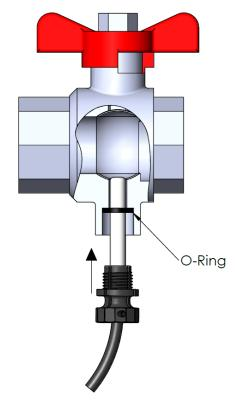
The guide of the O-ring is used for sliding the O-ring into place after which the sensor can be pushed as far as it will go.
