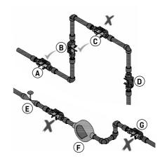
In order to avoid cavitation, the back pressure at the flow sensor (the pressure at the flow sensor outlet) must be minimum 1.5 bar at  $q_p$  (nominal flow) and minimum 2.5 bar at  $q_s$  (maximum flow). This applies to temperatures up to approx. 80 °C.
